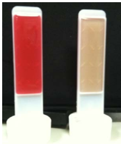
Figure 3. Representative dip-slide with double agar sides free of microbial contamination. This dip-slide was used to test the LoxaSperse dispersion for up to 24 h of environmental exposure.
